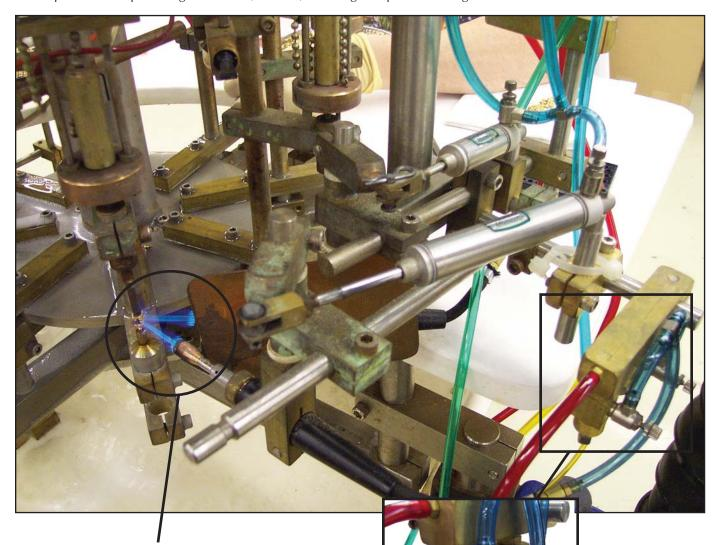
The machine consists of a rotating center carousel with eight stations. The individual components of each slip-on fitting are loaded into clamp fixtures mounted on the carousel. The carousel indexes to each of the process stations: load, heat, cool, quench, and unload. The control and timing of the machine is accomplished using Clippard modular valves and brass limit
